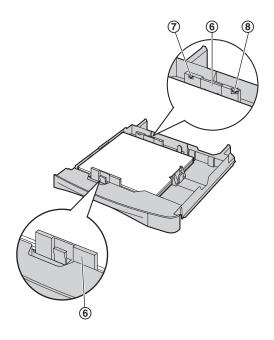
5 Insert the standard input tray to the unit, lifting the front part of the tray. Then push it completely into the unit.
